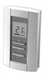
The ZonePRO® thermostats are for low-voltage pressure-dependent variable air volume (VAV) applications. ZonePRO® can also be used for hydronic perimeter heating/cooling and bypass box with or without reheat. The four models cover modulating applications, floating applications and applications that require up to two additional outputs for reheat.
