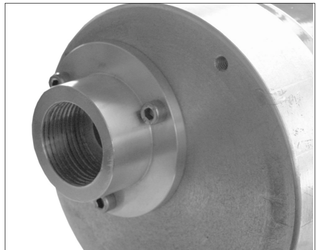
Fig. 9. Mounting the C7061F detector
