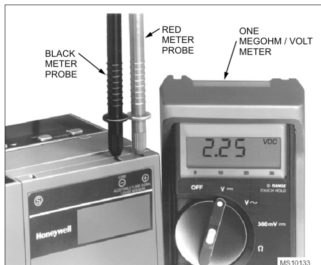
Fig. 11. Measuring voltage flame Signal with 7800 SERIES controls
