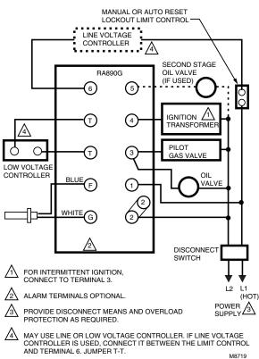
The use of manual reset limits is desirable with the RA890G to prevent the system from cycling off the high limit and to assure that the condition that causes the limitation is detected as soon as possible.
