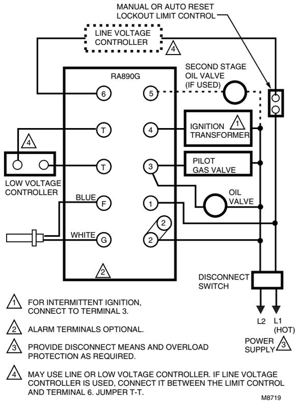
The use of manual reset limits is desirable with the RA890G to prevent the system from cycling off the high limit and to assure that the condition that causes the limitation is detected as soon as possible.
