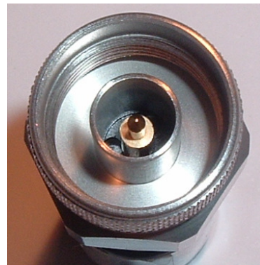
Figura 13b: Conductor externo sin ranuras (slotless)
