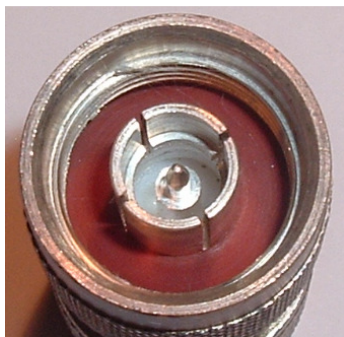
Figura 13a: Conductor externo ranurado (slotted)
